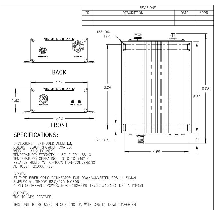
NOTES: NOMINAL 20 mA PULLED FROM GPS RECEIVER. WHEN FAULT OCCURS, AN ADDITIONAL 40 mA IS PULLED TO INDICATE FAULT TO THE RECEIVER.
