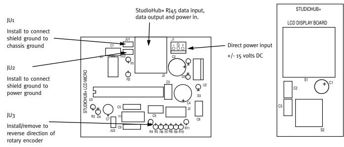
This board must be used in conjunction with the LCD display board.
